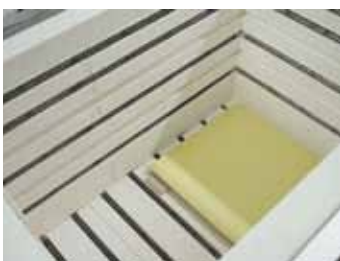
Firing chamber with heating from 5 sides
