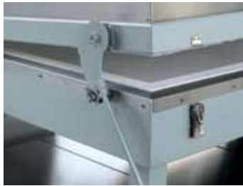
Locking device provides for defined hood opening in different positions and accelerated cooling
