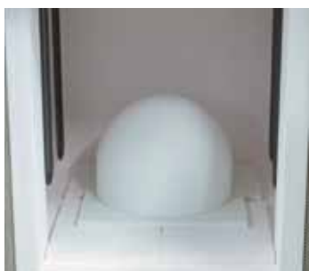
Gastight retort with gas injection through the furnace floor
