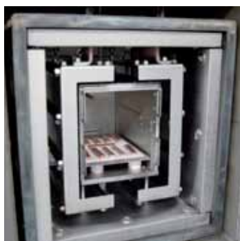
Heat treatment of copper bars under hydrogen in VHT 08/16 MO
