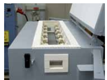
Furnace chamber of the GR 1300/13 with second door as additional equipment
