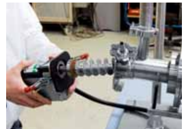
Screw-conveyor with adjustable speed
