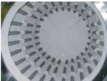
Heating from outside around the retort in models NRA .../09 and NR .../11
