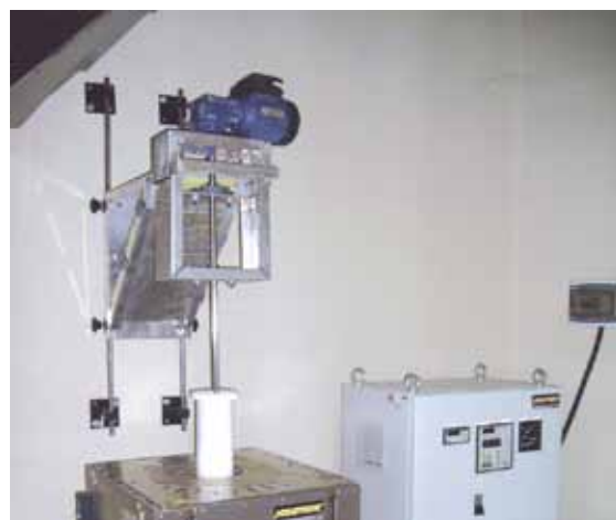
RHTV 120/300/15 integrated in a tensile strength testing machine
