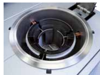
Cylindrical retort with tungsten heating
