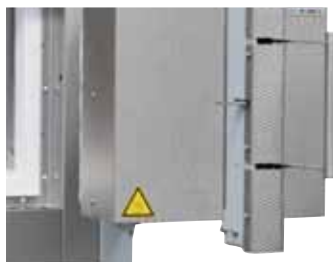
Parallelly guided door provides for heat protection of the operator
