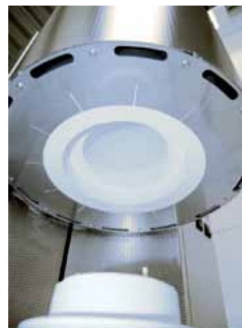
Plasma ceramic retort for protection of the heating elements and to avoid charge contamination [in the LHT 02/16 LBR]
