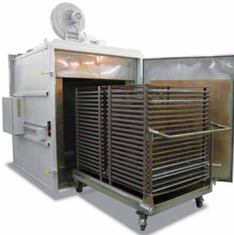
N 2380/55 HAC air circulation furnace in customized version with charging cart and shelves made of 1,4828 stainless steel
