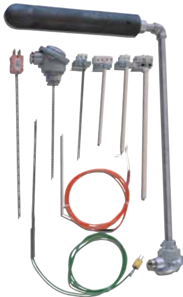
Calibrated thermocouples in various designs
