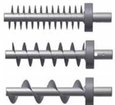
Screw-conveyors with different pitches for the adaption to the charge
