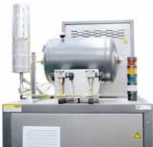
Nitrogen emergency purging and exhaust gas torch for hydrogen version
