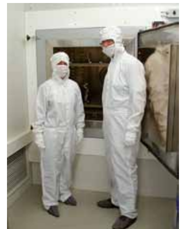
Industrial oven N 250/65 HAC with particle-free oven chamber. For charging, furnace door is located in cleanroom, class 100, furnace chamber in greyroom behind.
