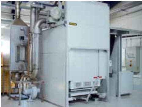
Combi chamber furnace system with catalytic afterburning for debinding and sintering
