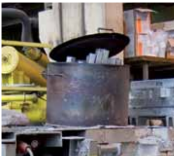
Charging funnel for ingots
