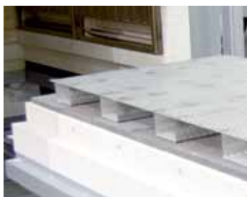
Charge support in a circulating air bogie hearth furnace for 850 °C
