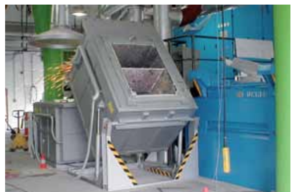
Tilting furnaces for magnesium K 1500/75 S with 1500 liters crucible volume
