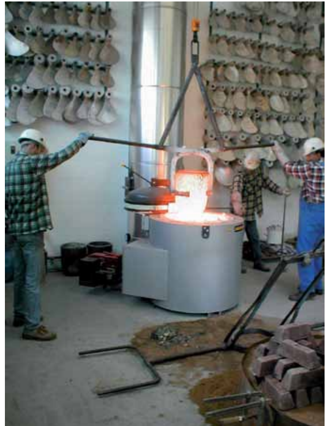
TB 40/14 with crucible pulling device
