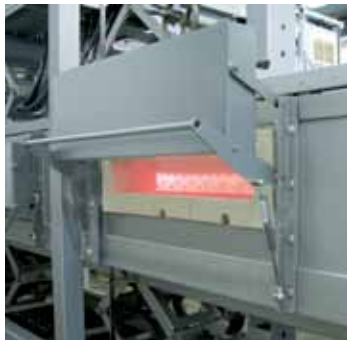
Service flap door at furnace side
