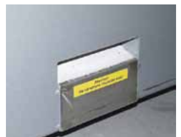
Emergency outlet for the safe draining of melt in case of crucible breakage
