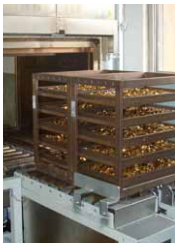
Continuous belt furnace for heat treatment of rivets
