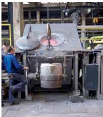
Charging of transport ladle with K 360/12
