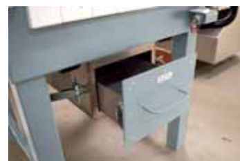
Drawer for collection of liquid wax
