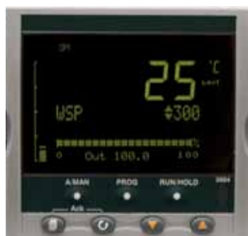
Compact controller Eurotherm 3504
