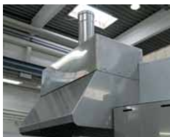
Exhaust hood above charging opening
