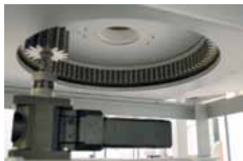
Gear rim drive under the furnace
