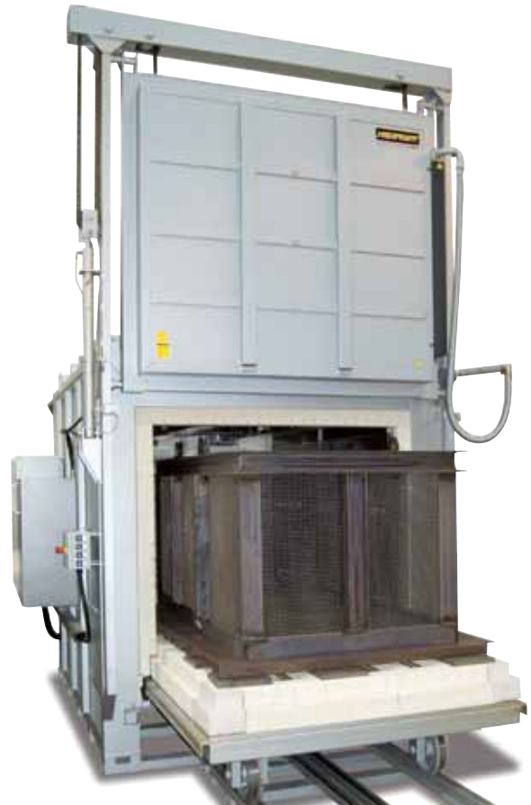
W 4000/60AS with charging basket made of 1.4828
