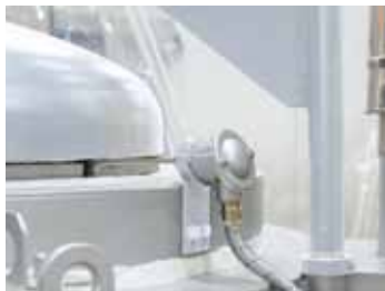
Thermocouple for melting bath control
