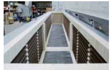
Furnace chamber S 5120/GS with device for an insulating plate in order to divide the furnace chamber
