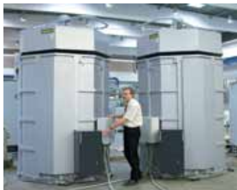
2 x S 3570/65 AS for solution annealing
