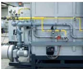
Chamber furnace with gas supply system
