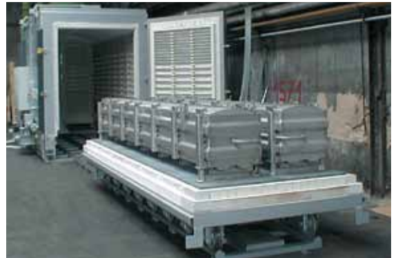
Bogie hearth furnace with gas supply system
