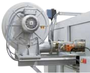
Cooling fan for accelerated cooling
