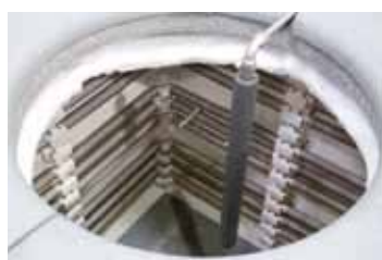
Design of a holding furnace with bath control system containing thermocouples for the melt, the furnace chamber and the over-temperature limit controller
