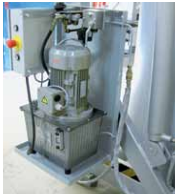
Hydraulic system with flame resistant hydraulic fluid
