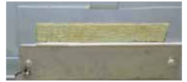
Crucible breakage alarm device under the emergency outlet of a melting furnace
