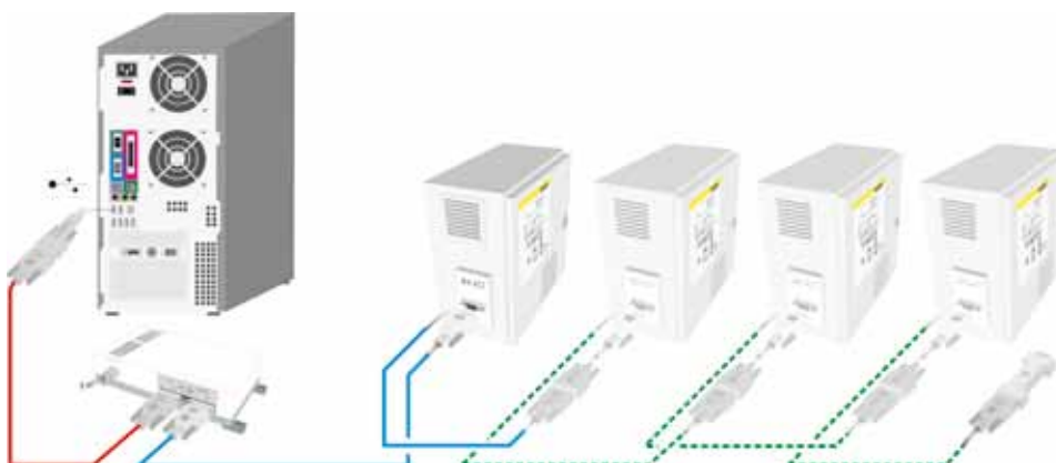
Extendable for connection of up to 16 furnaces
