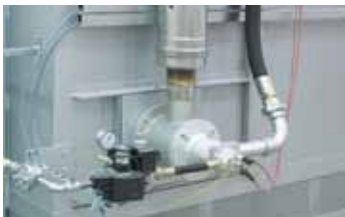
Gas burner positioned along the furnace side
