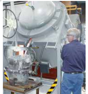
KB 240/12 for melting aluminum alloys
