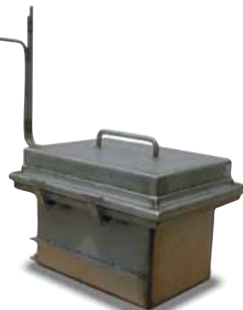
Annealing box with protective gas inlet and outlet, constructed for evacuation at ambient temperatures
