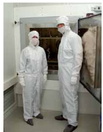
Industrial oven N 250/65 HAC with particle-free oven chamber. For charging, furnace door is located in cleanroom, class 100, furnace chamber in greyroom behind.
