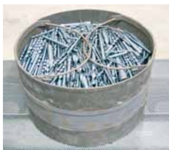
Blueing of drills in water steam atmosphere in a furnace of the NRA range
