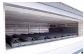
Furnace chamber with supporting rails for metal trays
