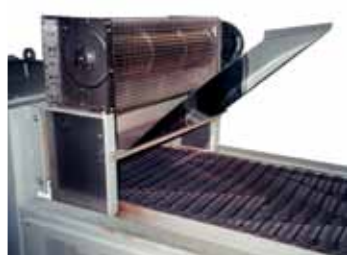
Cooling facility at discharge of a continuous belt furnace
