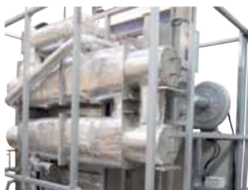
Counterflow heat exchanger for the air circulation chamber furnace N 2560/26 ACLS
