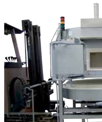
Furnace floor can be lowered for maintenance purposes
