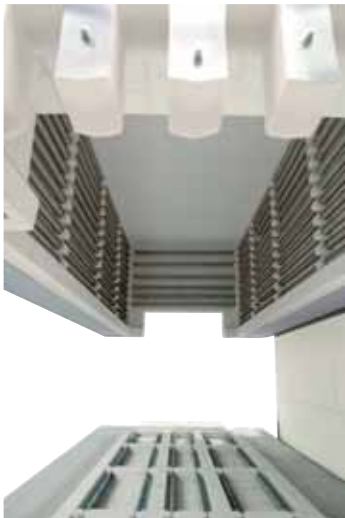
Lift-top furnace with recesses for extending charges
