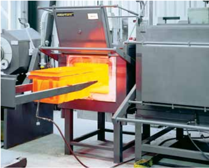
Powder nitriding in an annealing box
