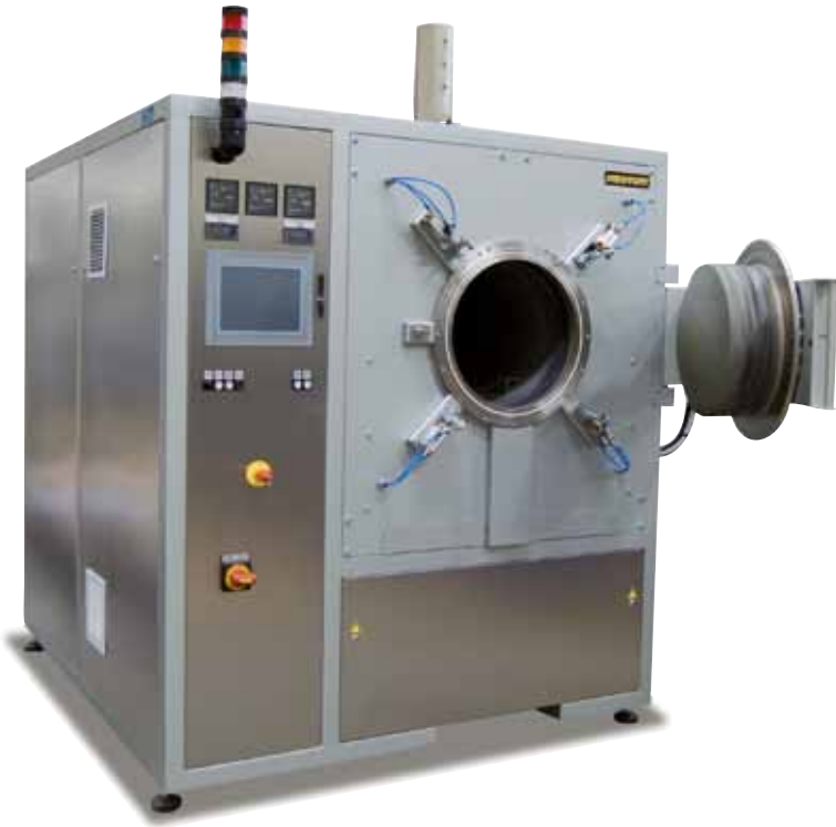
NR 50/11 with gas supply package and safety system for hydrogen
