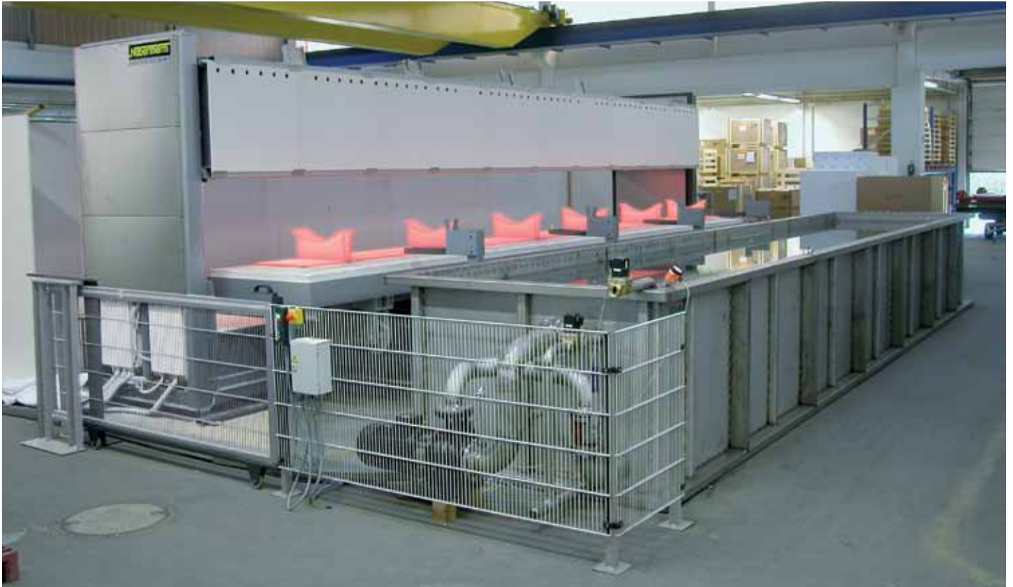
Annealing system with top-hat furnace H 4263/12S and water bath
