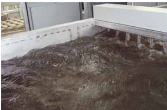
Powerful circulation of quenching medium
