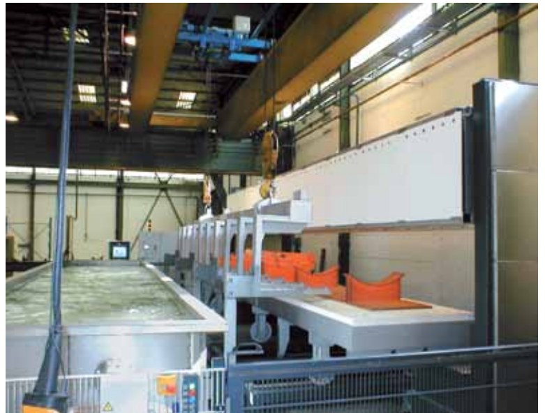
Manual heat treatment system for hardening of steel rods, see page 59
