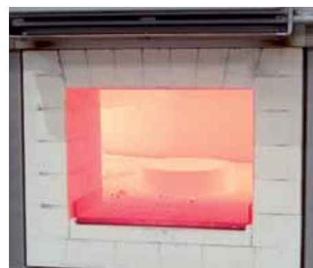
Pre-heating of steel rings for forging
