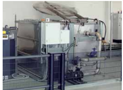
quench tank with water integrated in a heat treatment system for aluminium
