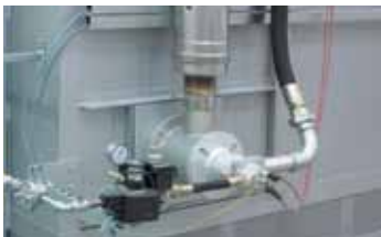
Gas burner positioned along the furnace side
