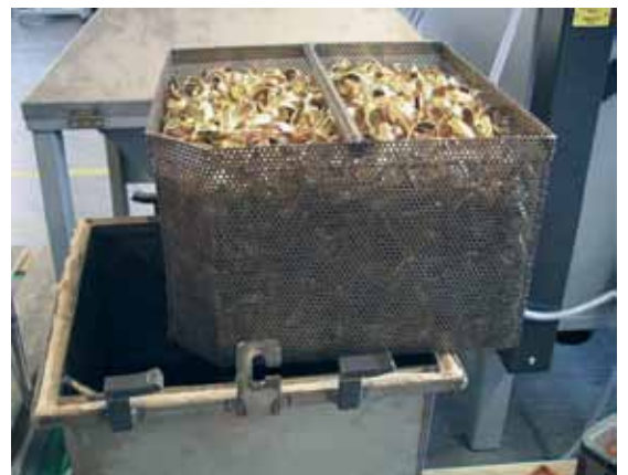
Bulk material bright annealing in an annealing box with evacuation facility
